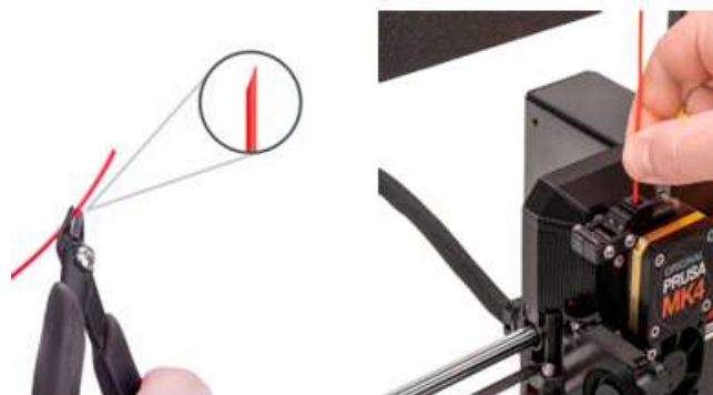
Figure 4 Loading the PLA filament into the Nexttruder
